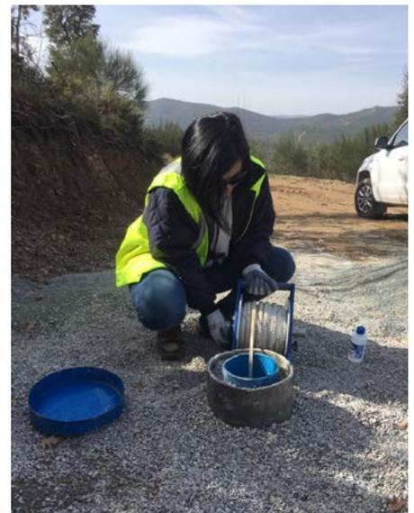
*Water level monitor in a borehole*
