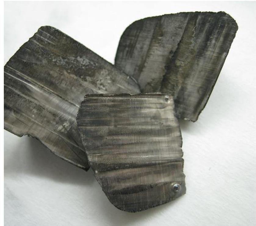
Lithium ingots with a thin layer of black nitride tarnish
