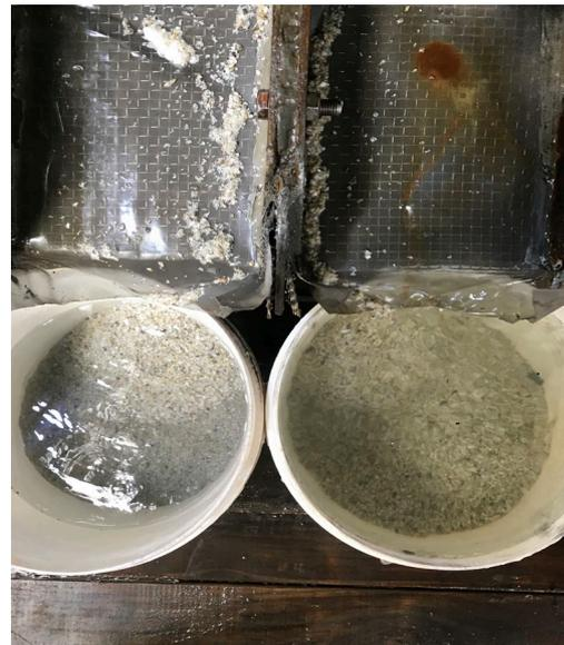
**Nagrom DMS100 Test Plant - Left Bucket SG2.65 Float (Waste Material) Right Bucket SG2.65 Sinks (Spodumene Concentrate)**
