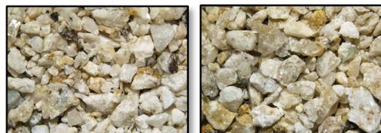
**Left Photo SG2.65 Float (Waste Material) Right Photo SG2.65 Sinks (Spodumene Concentrate)**
