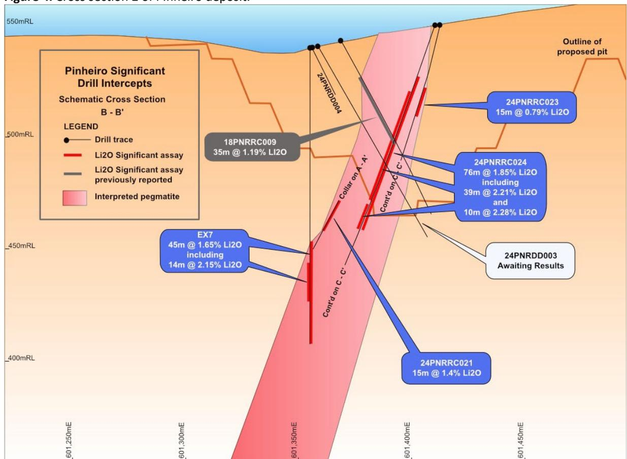
**Figure 5.** Cross section 3 of Pinheiro deposit.
